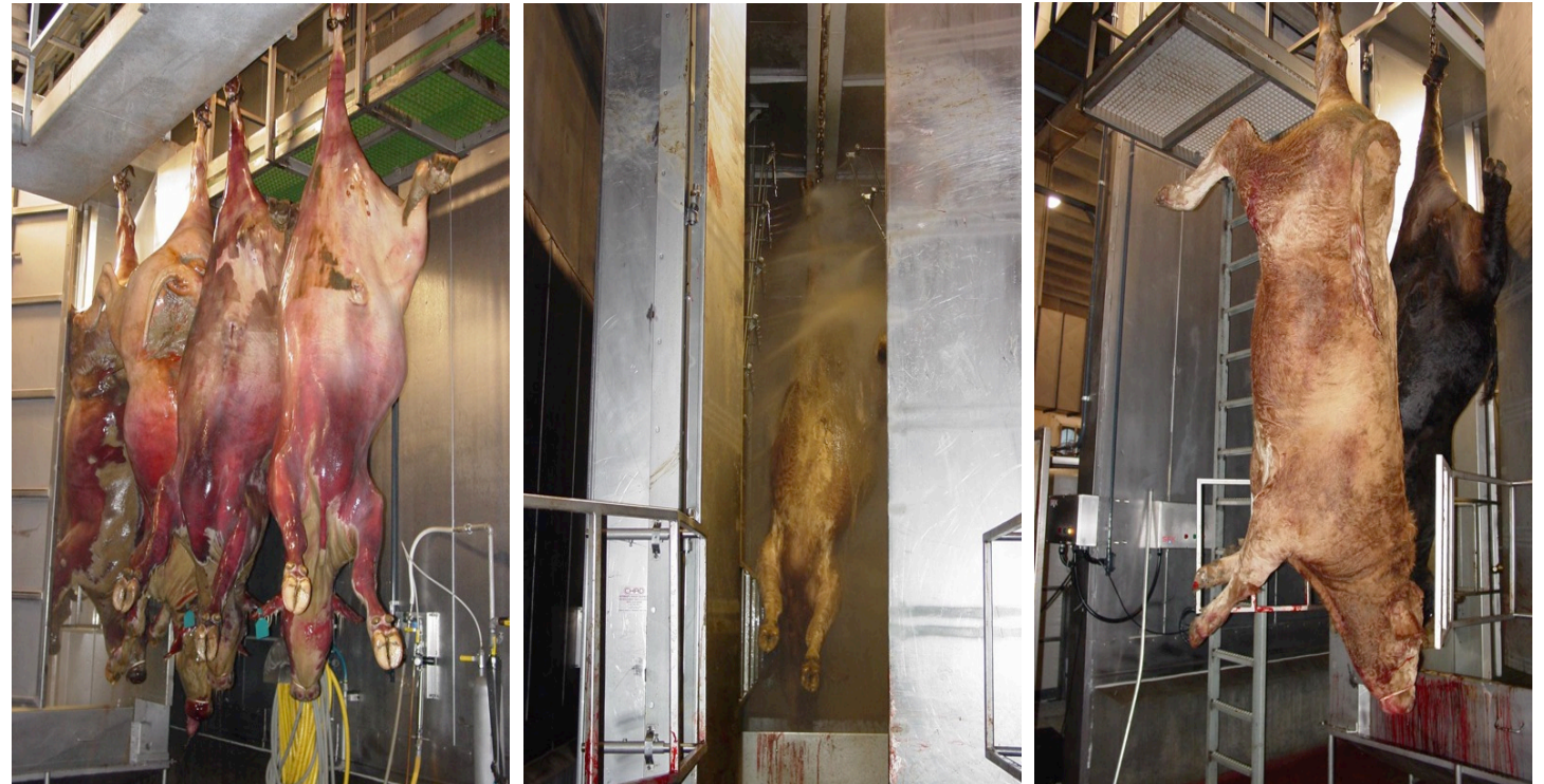
Chemical dehairing consists of washing hide-on carcasses with a solution of sodium sulfide, followed by hydrogen peroxide to neutralize and water to rinse.
