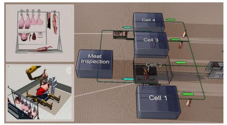
Overview of the initial MFC concept (bottom-left) and a rack (top-left). The concept (right) enables parallel rather than serial task-execution in abattoirs for greater flexibility, scalability and robustness at all volumes of production.
